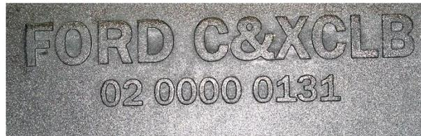
**Note:** *The tank body has the above identification on its top. Please check to be sure the tank is properly identified as the one to fit your vehicle.*
